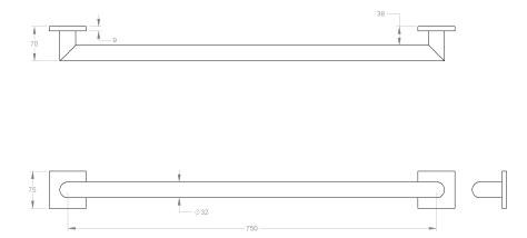
ICO grab bars can support loads of up to 440lbs if properly installed in compliance with ADA requirements.
